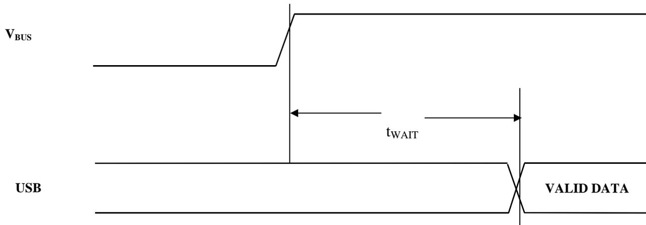
The module resets automatically at power-up and initializes to the same conditions as after the Reset Command.
